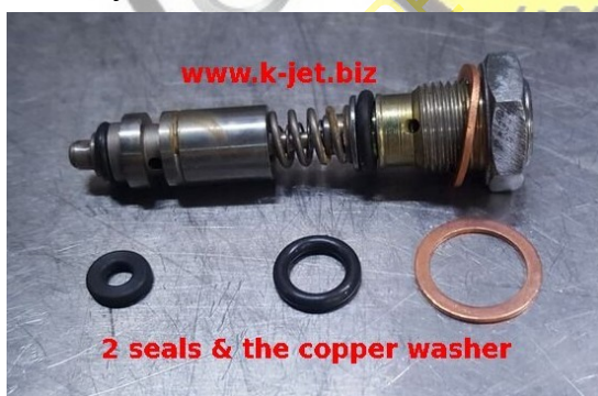
Late System Pressure valve (type 3)
