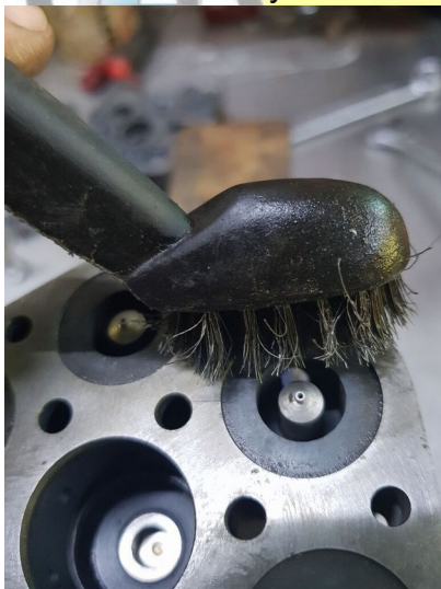
cleaning around the nozzle
